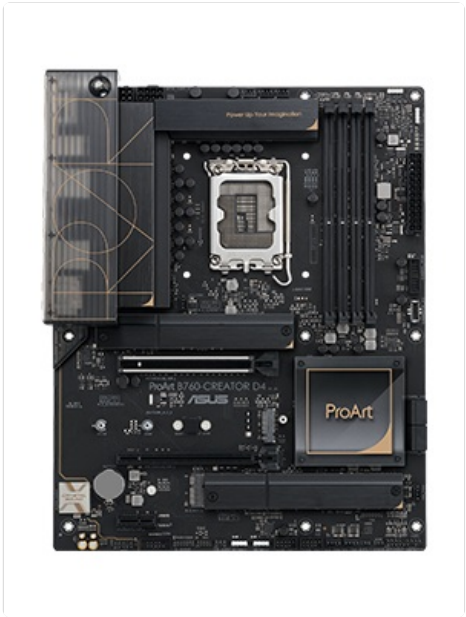
Image Description: A detailed view of the LGA 1700 CPU socket on the motherboard, showing the intricate pin array and the CPU retention mechanism. This socket is compatible with 12th and 13th Generation Intel Core processors.
