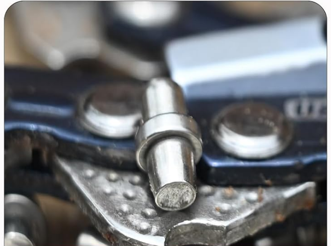
Platinum Rivet Reduce wear and chain stretch
