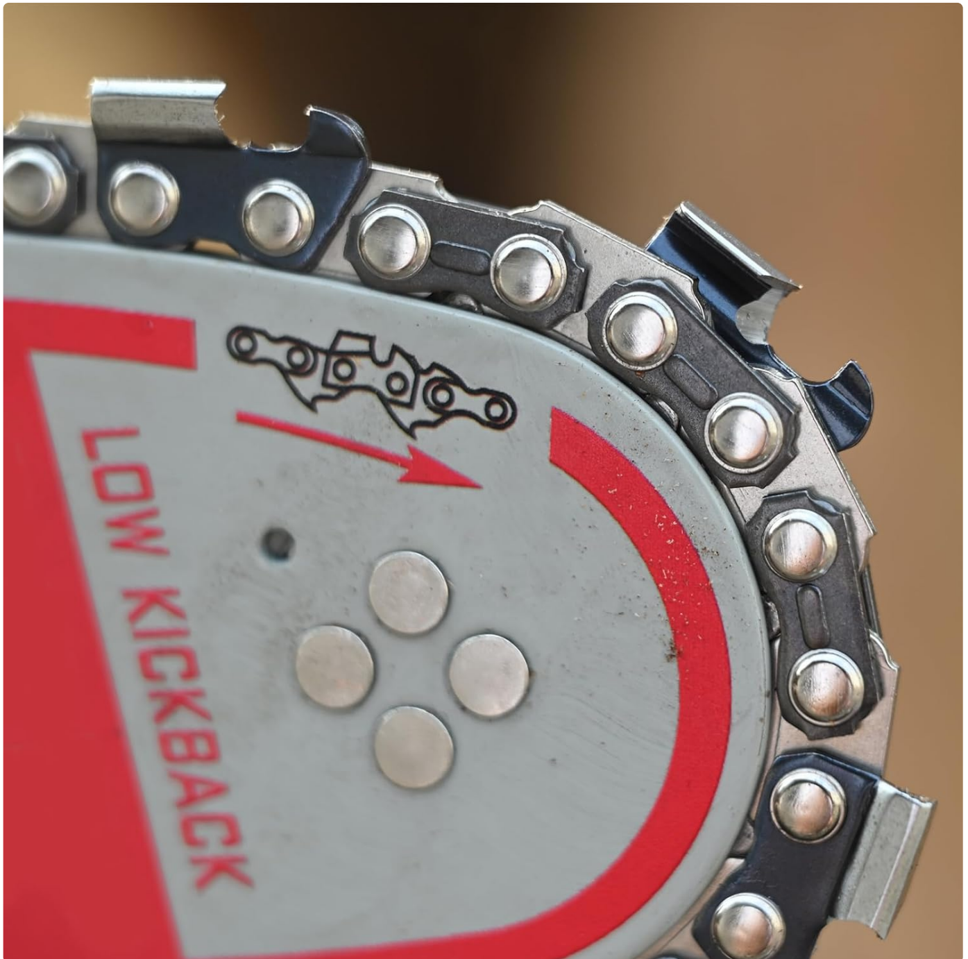
Figure 4: Correct chain orientation on the guide bar.
