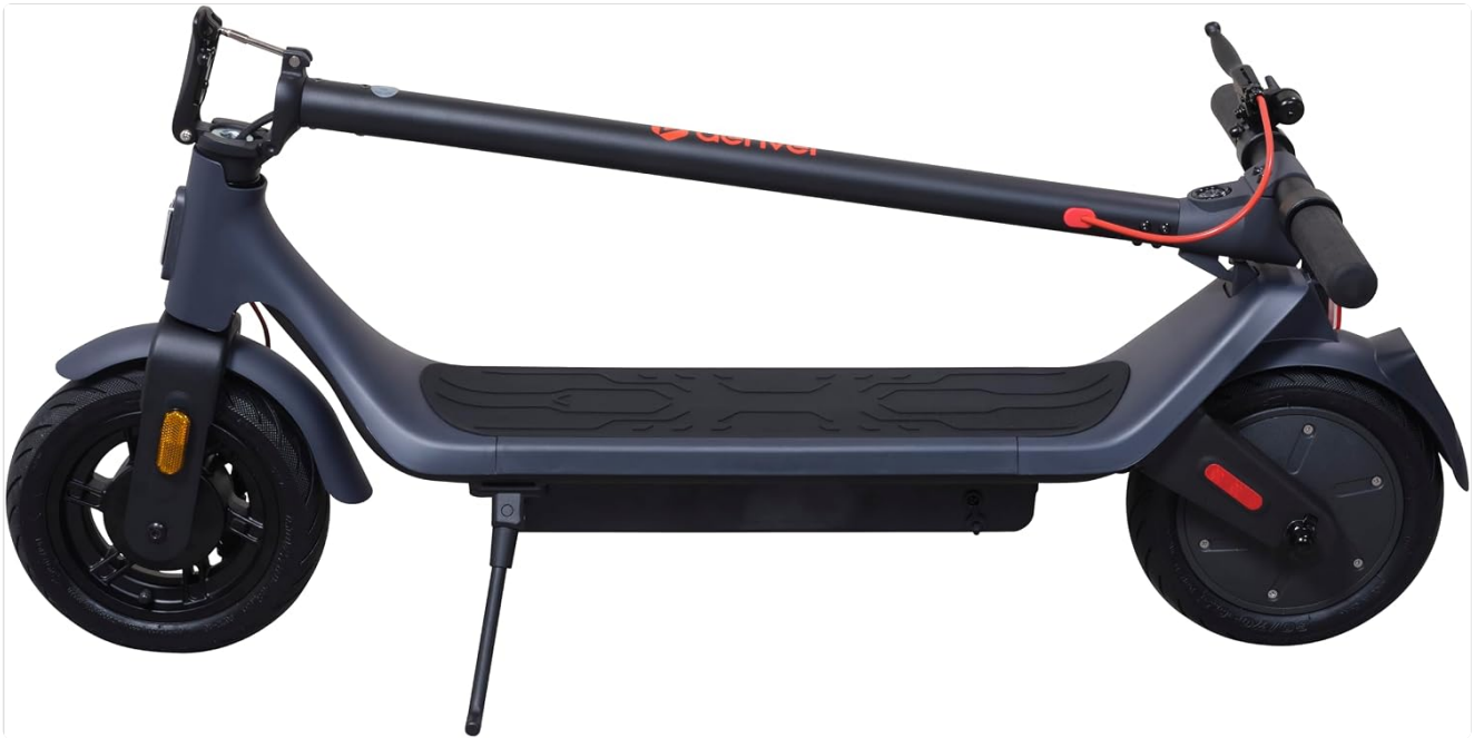
Figure 7: Scooter in folded position for compact storage.
