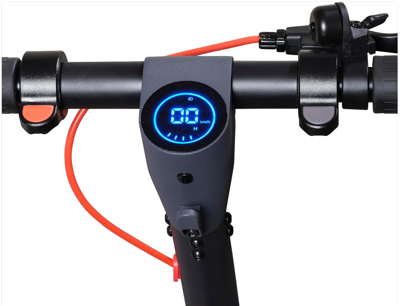
Figure 4: Handlebar display showing operational information.
