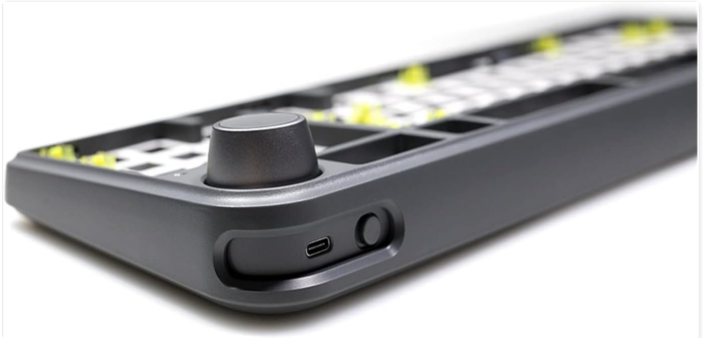
Figure 2: Close-up view of the USB Type-C port and the power/mode switch located on the side of the keyboard.
