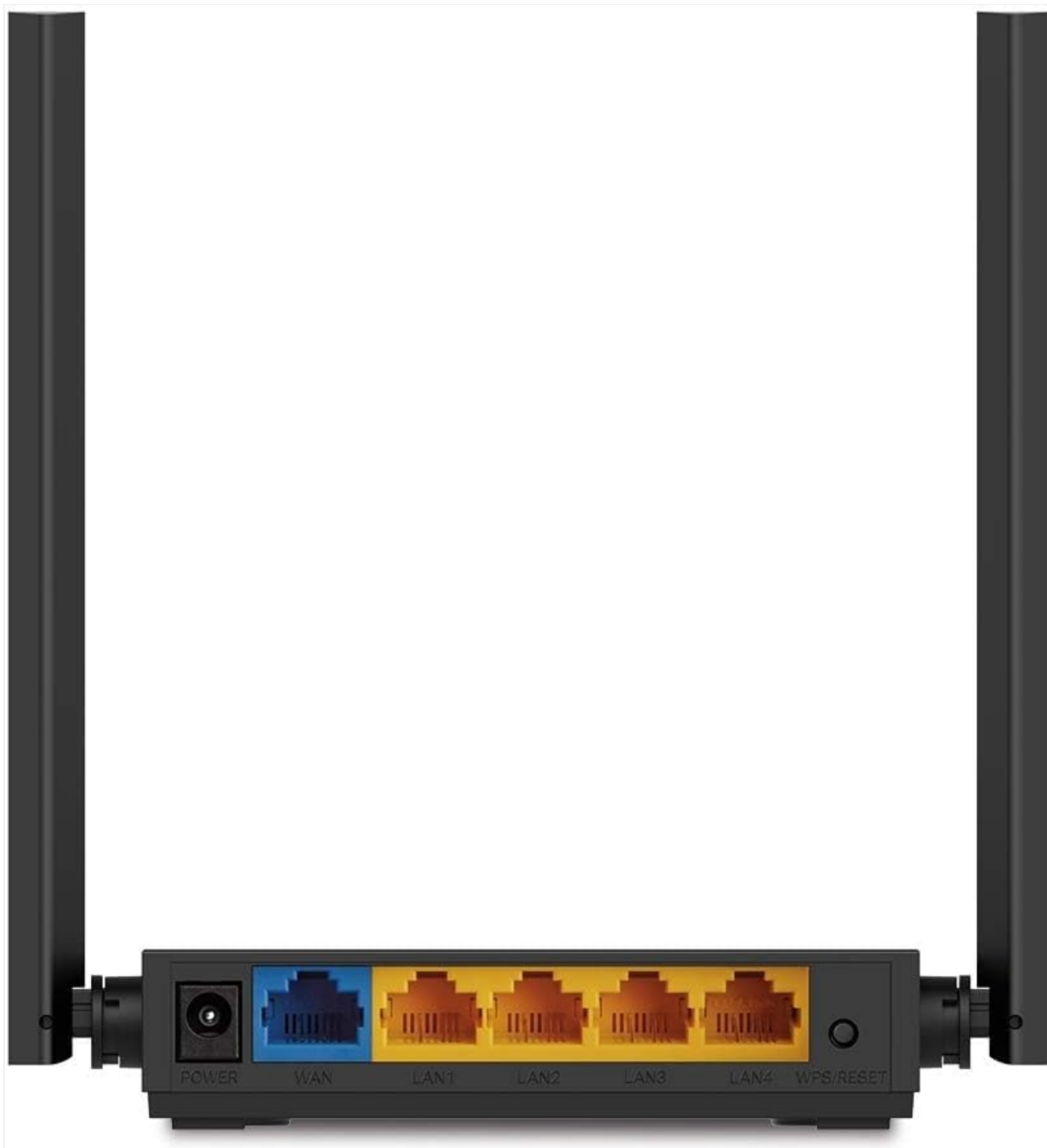
Figure 1.2: Rear panel of the Archer C54, displaying connectivity ports and buttons.
