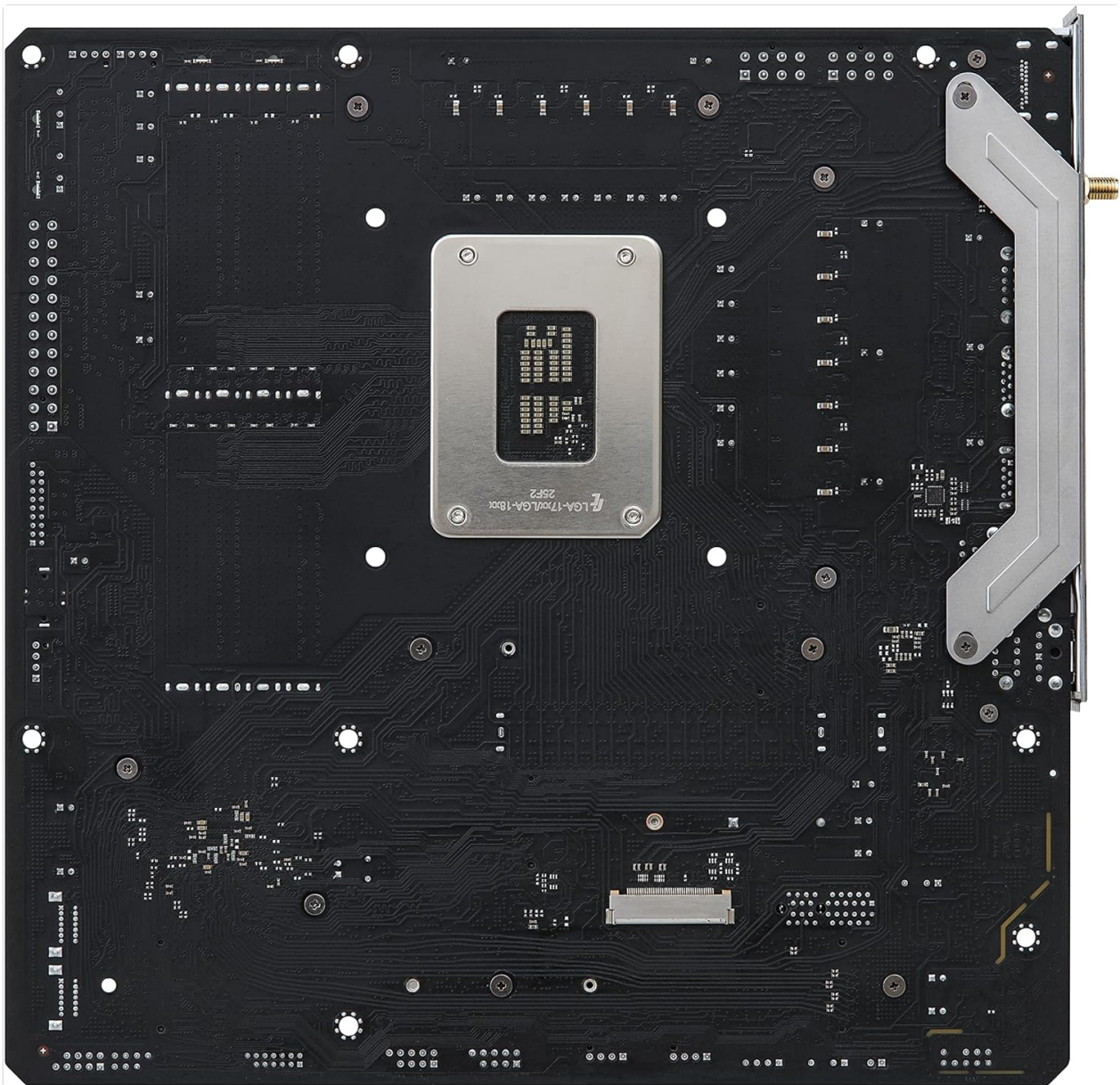
Image 3.2: Rear view of the motherboard, showing the CPU socket backplate and general PCB layout.
