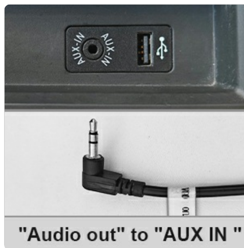
Figure 5.2: Audio Out to AUX IN Connection
