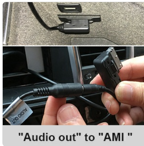
Figure 5.1: Audio Out to AMI Connection
