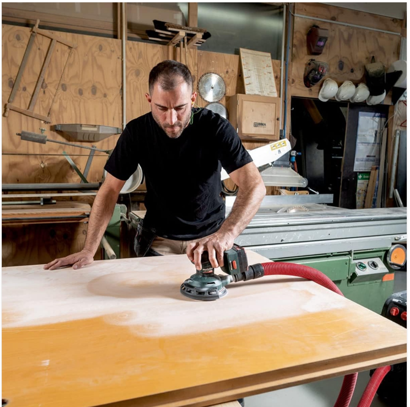
Image 5.3.2: Demonstrating the use of the sander with an external dust extraction system for cleaner operation.
