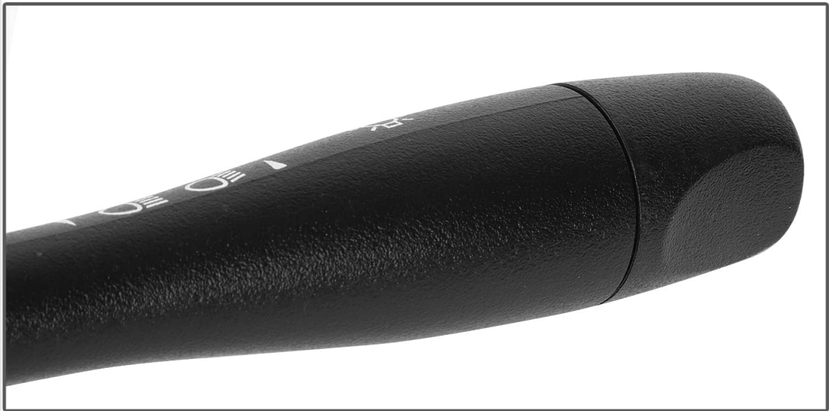
Image 4: Close-up view of the control stalk, showing the symbols for headlight settings (OFF, Parking, ON, AUTO) and turn signal arrows.
