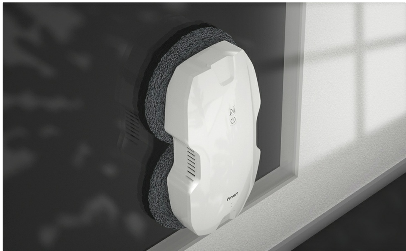
Image: An Fmart window cleaning robot actively cleaning a large window, demonstrating its operation.
