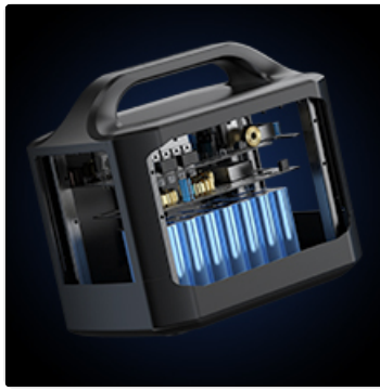
Figure 2: Internal view of the power station, highlighting the battery pack and circuit board. Do not attempt to open the casing.
