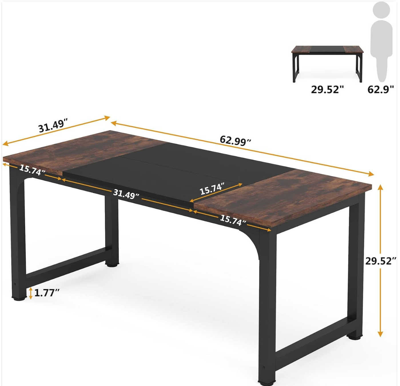
Figure 2: Desk dimensions and key measurements for assembly.
