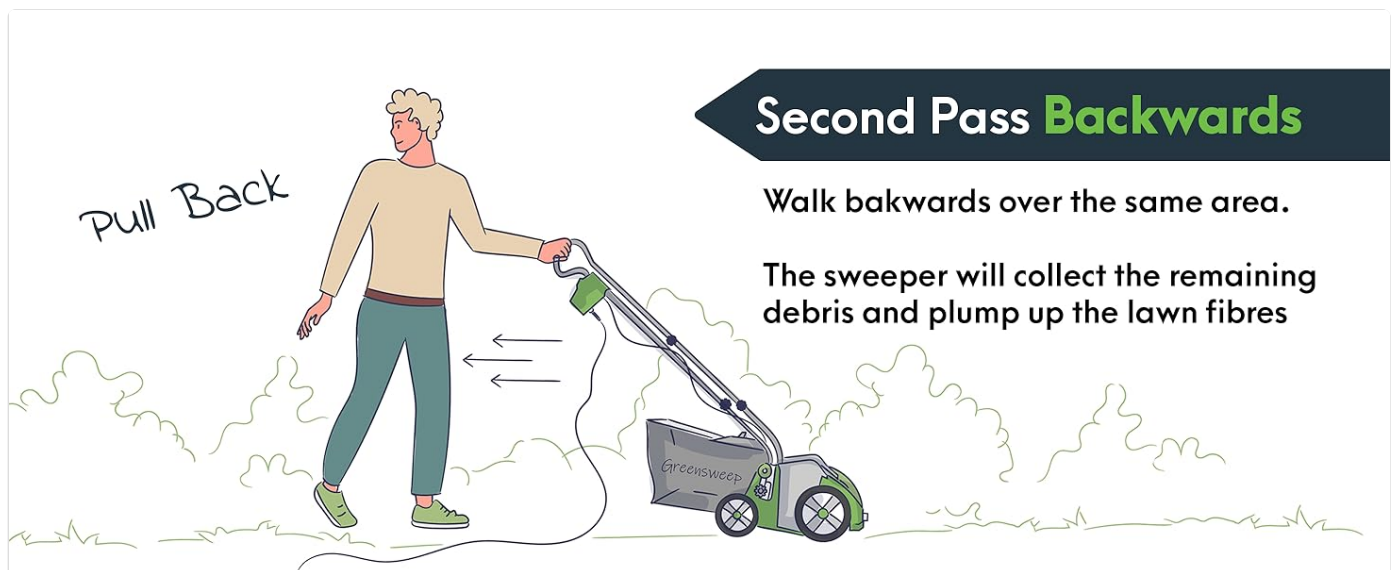
Figure 5: Illustration of the second pass, pulling the sweeper backward.
