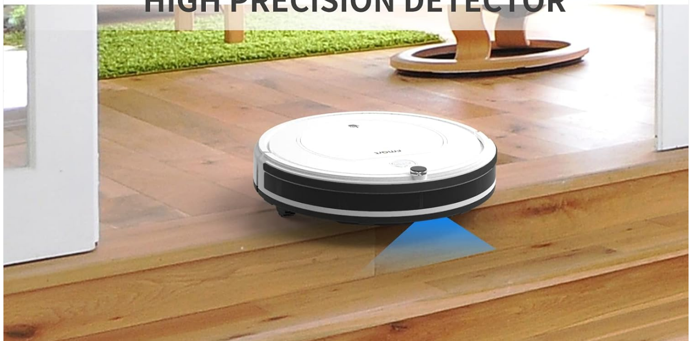
Image 4.4: The robot's high-precision detectors enable it to sense and avoid obstacles and prevent falling down stairs.
