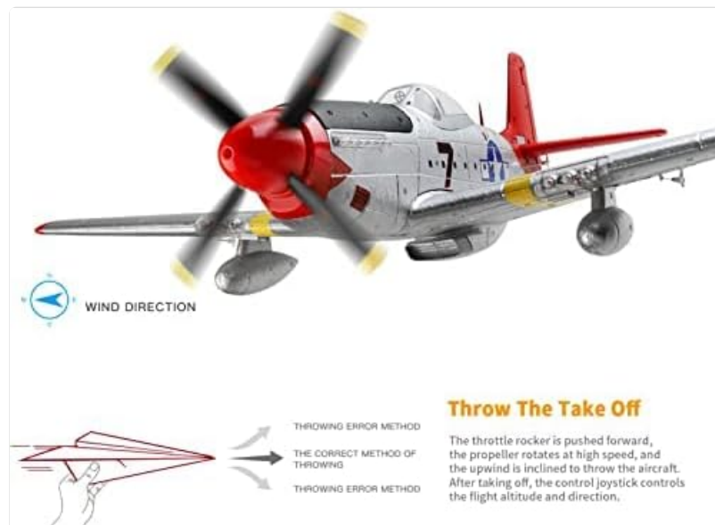
Figure 9: Diagram illustrating the correct method for hand launching the aircraft.
