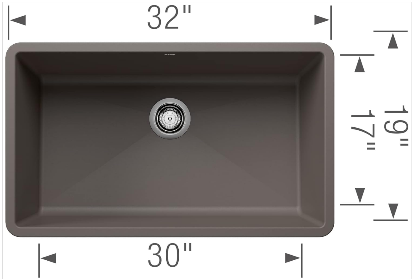
Image: Technical drawing illustrating the dimensions of the BLANCO PRECIS SILGRANIT sink, including its 32" L x 19" W overall size and 30" L x 17" W bowl dimensions.
