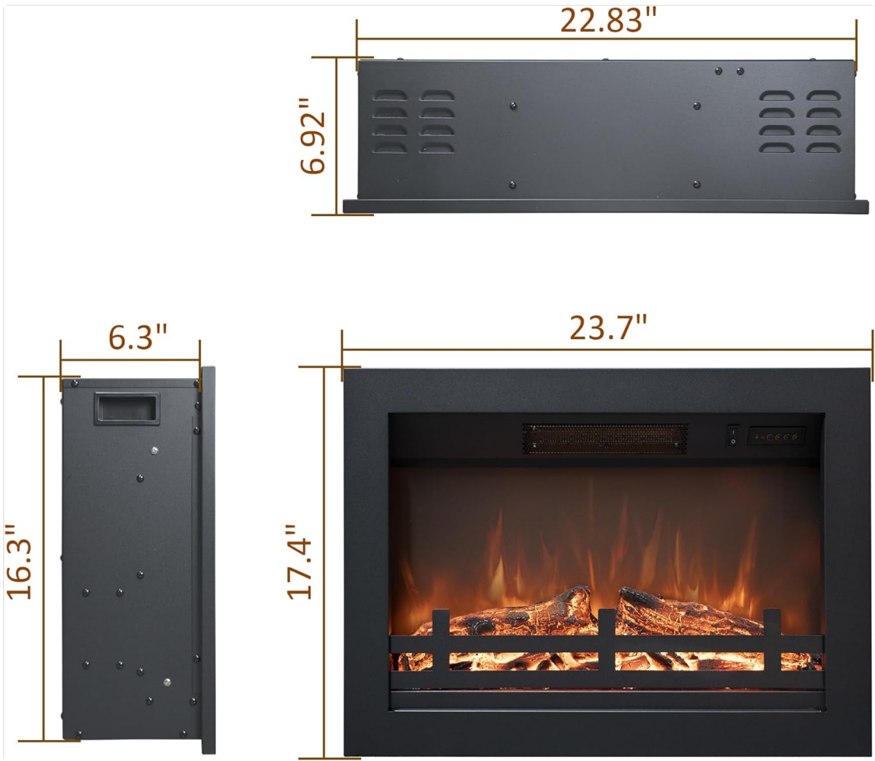
Image 4.1: Product dimensions for installation planning.
