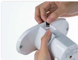
Figure 5.11: The camera supports local storage via an SD card (not included).
