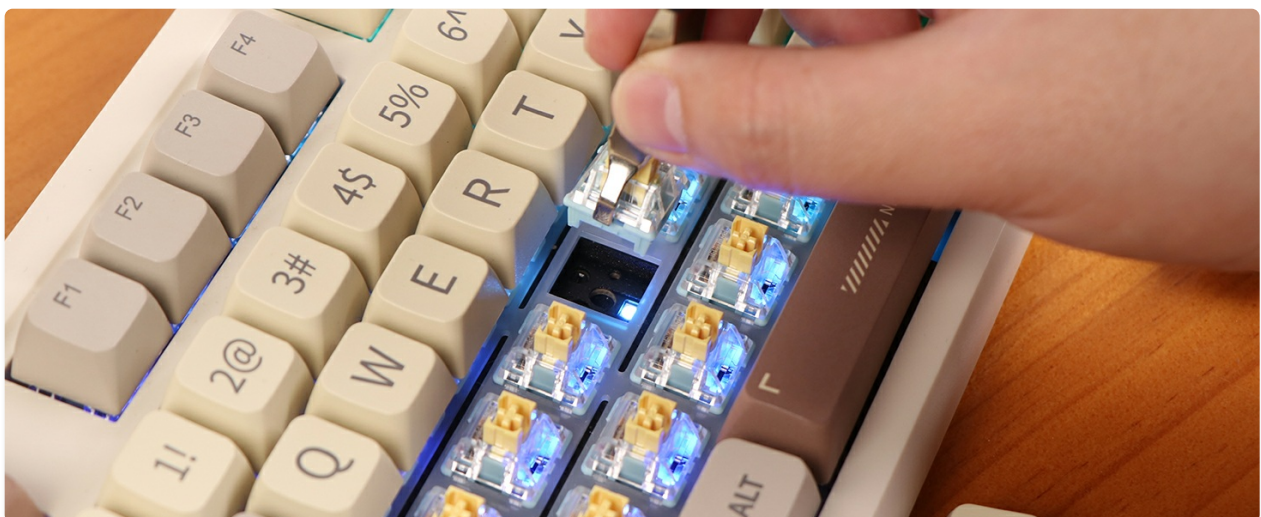
Image 5.2: A user removing a switch from the EPOMAKER RT100 keyboard, illustrating the hot-swappable feature.
