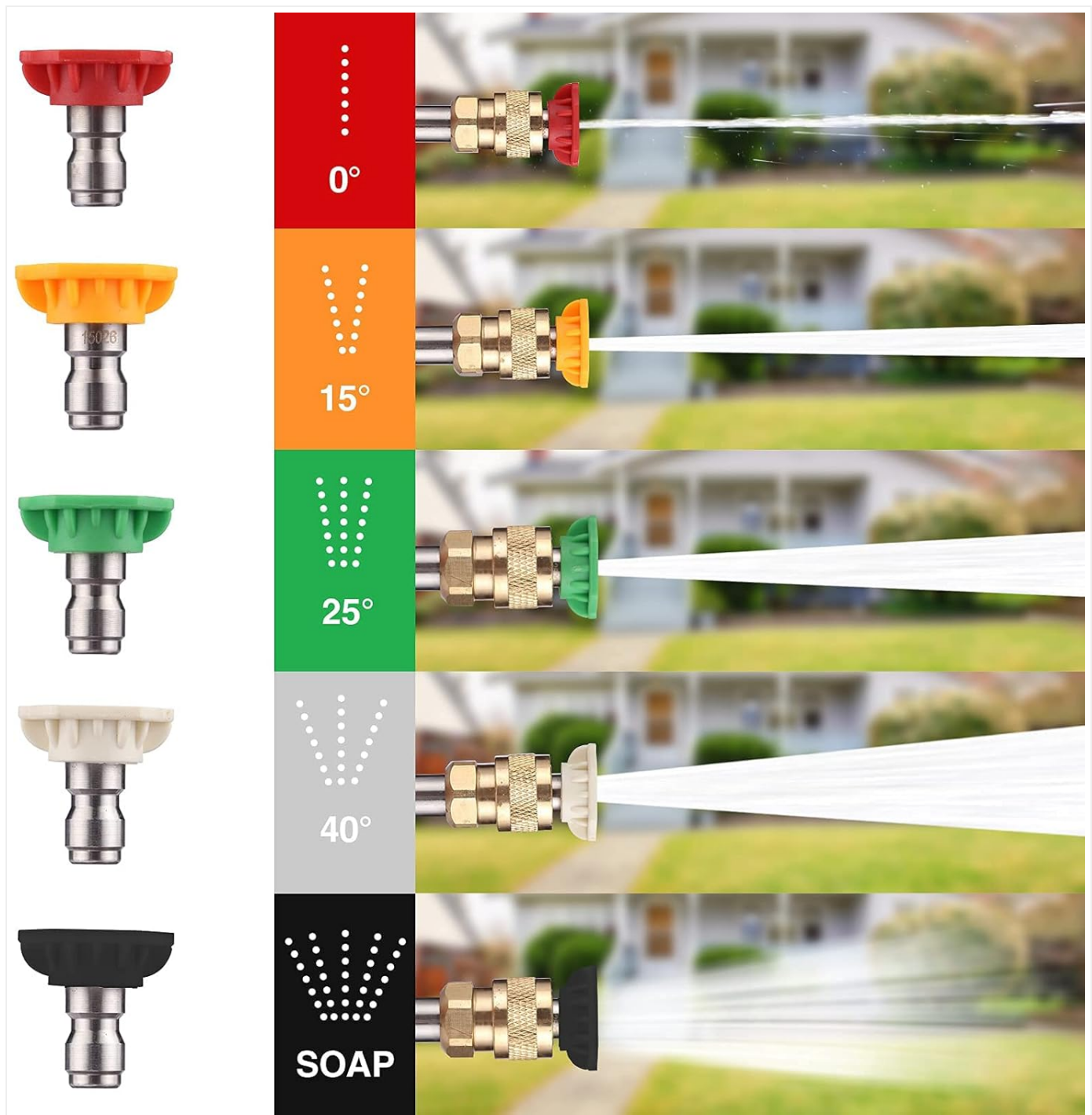
Figure 5.1: A visual guide to the five quick-connect nozzles included: red (0° for concentrated stream), yellow (15° for intense cleaning), green (25° for general cleaning), white (40° for wide coverage), and black (SOAP for detergent application).
