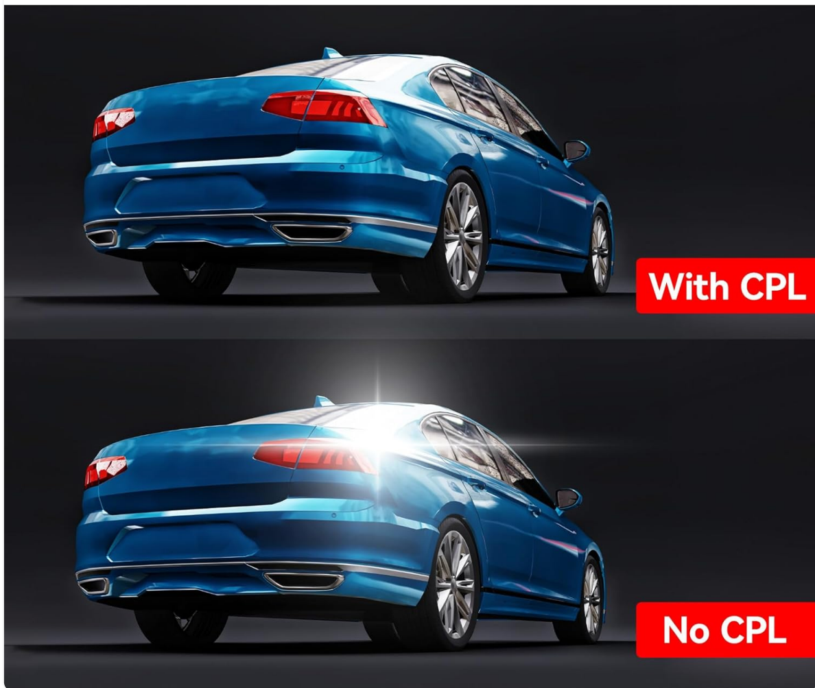
Figure 4.2: Effect of the CPL filter on reducing reflections.
