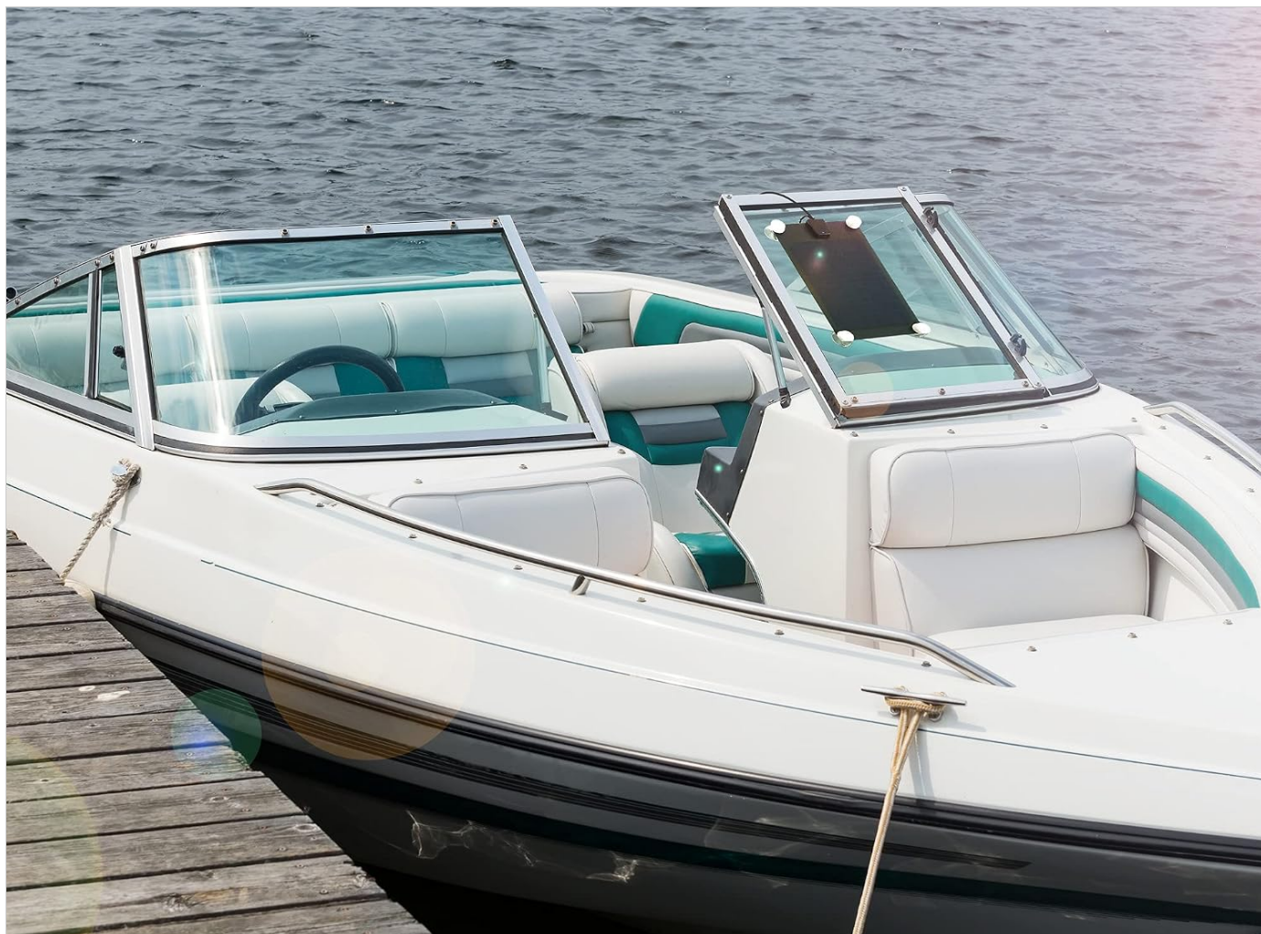
Image 2: A Nature Power semi-flexible solar panel installed on the windshield of a boat, demonstrating a typical application.
