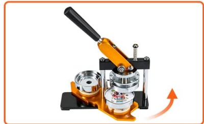
3. Align upper and lower dies
