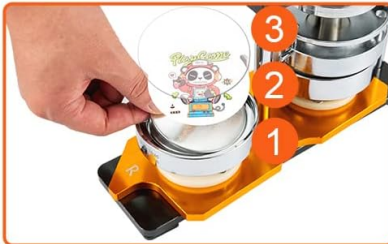
2. Put on tin up cover, paper and film
