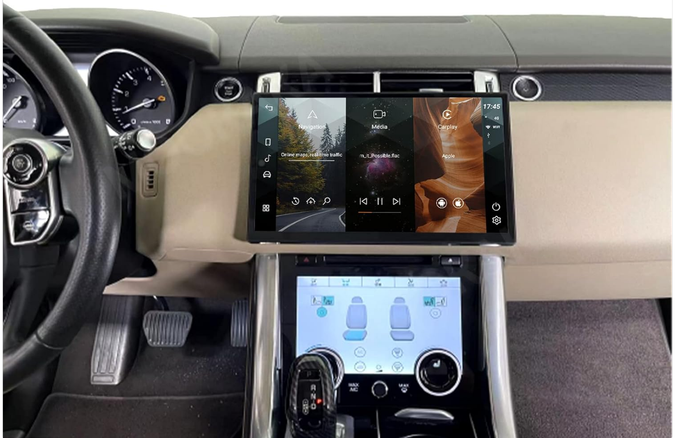
Figure 6.1: The 13-inch IPS touchscreen displaying a media player interface, highlighting its high resolution and visual clarity.
