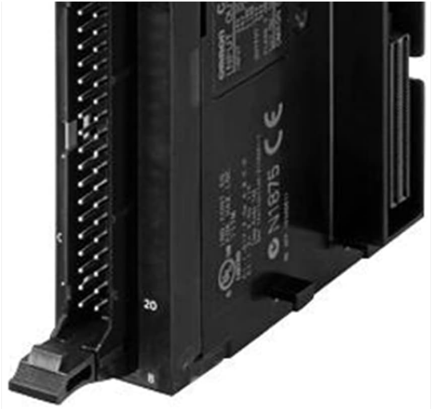
Figure 2: Detailed view of the CJ2M-MD211's input (IN) and output (OUT) terminal blocks, showing numerical labels for connections.
