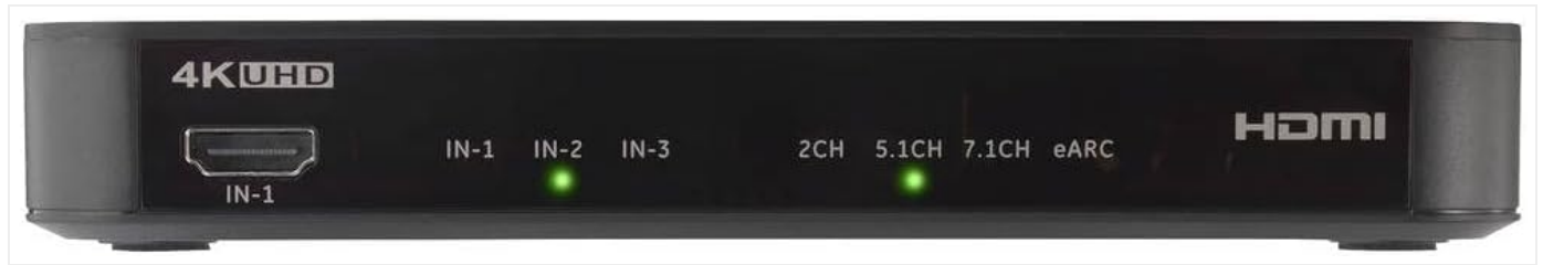
Figure 4.3: Detailed view of the front panel, showing the HDMI input indicators (IN-1, IN-2, IN-3) and audio mode indicators (2CH, 5.1CH, 7.1CH, eARC).
