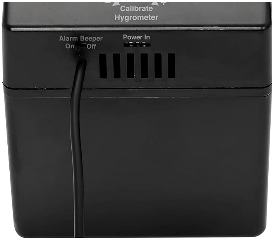
Image 6.1: Top view of the Hydra-LG main unit, highlighting the fan vents that require periodic cleaning.
