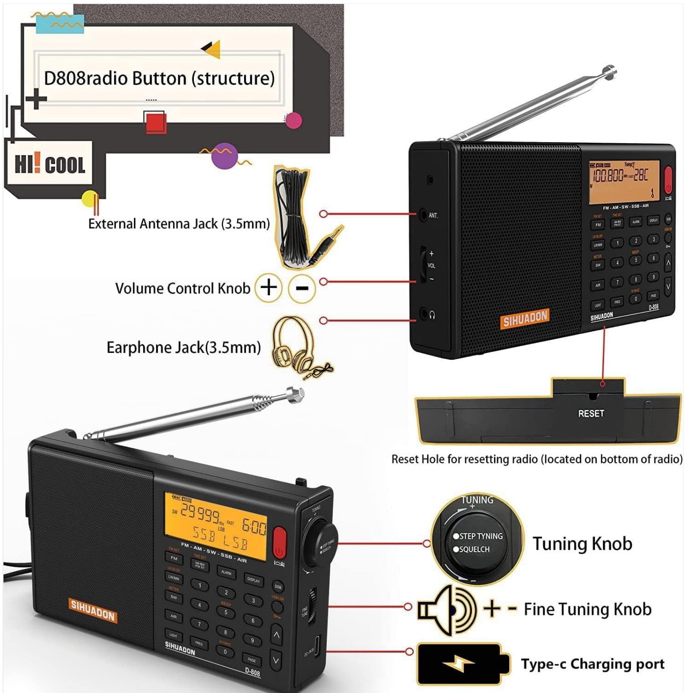
Figure 3.1: Detailed diagram showing the location of the external antenna jack, volume control knob, earphone jack, tuning knob, fine tuning knob, Type-C charging port, and reset hole on the SIHUADON D808 radio.
