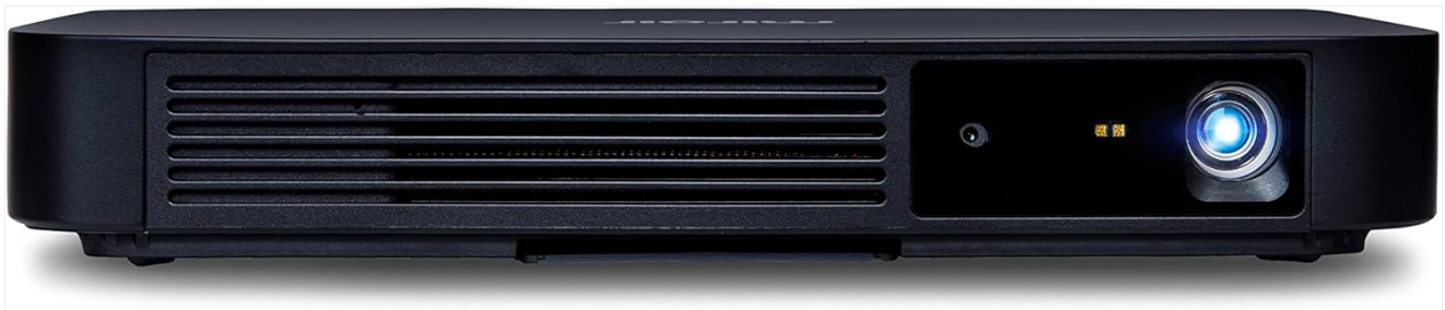
Figure 4.2: Front view of the Miroir M700S projector, highlighting the projection lens and ventilation grille.
