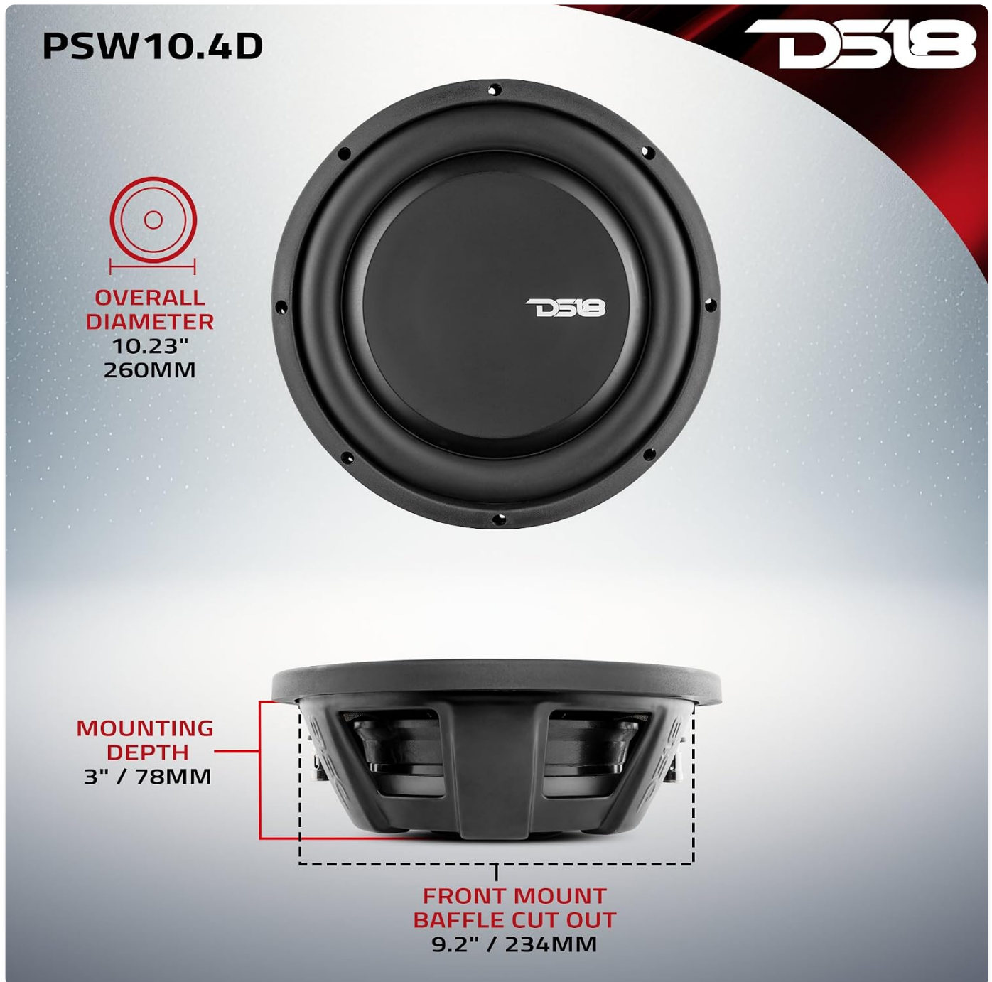
Image 2.1: Diagram illustrating the overall diameter (10.23" / 260mm), mounting depth (3" / 78mm), and front mount baffle cut-out (9.2" / 234mm) of the PSW10.4D subwoofer.
