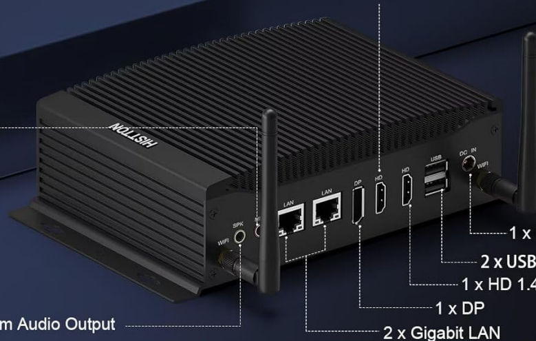
Image 3.2: Detailed view of the front and rear ports, including USB, HD, DP, LAN, COM, and GPIO.
