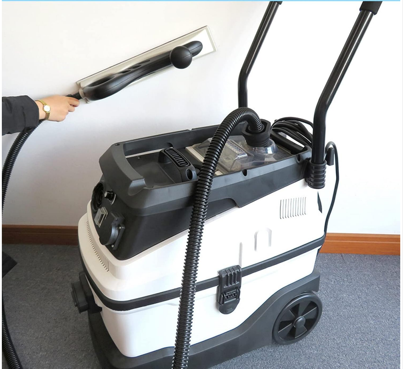
Figure 4: The hand sanding block connected via a hose to a dust extraction system for cleaner operation.
