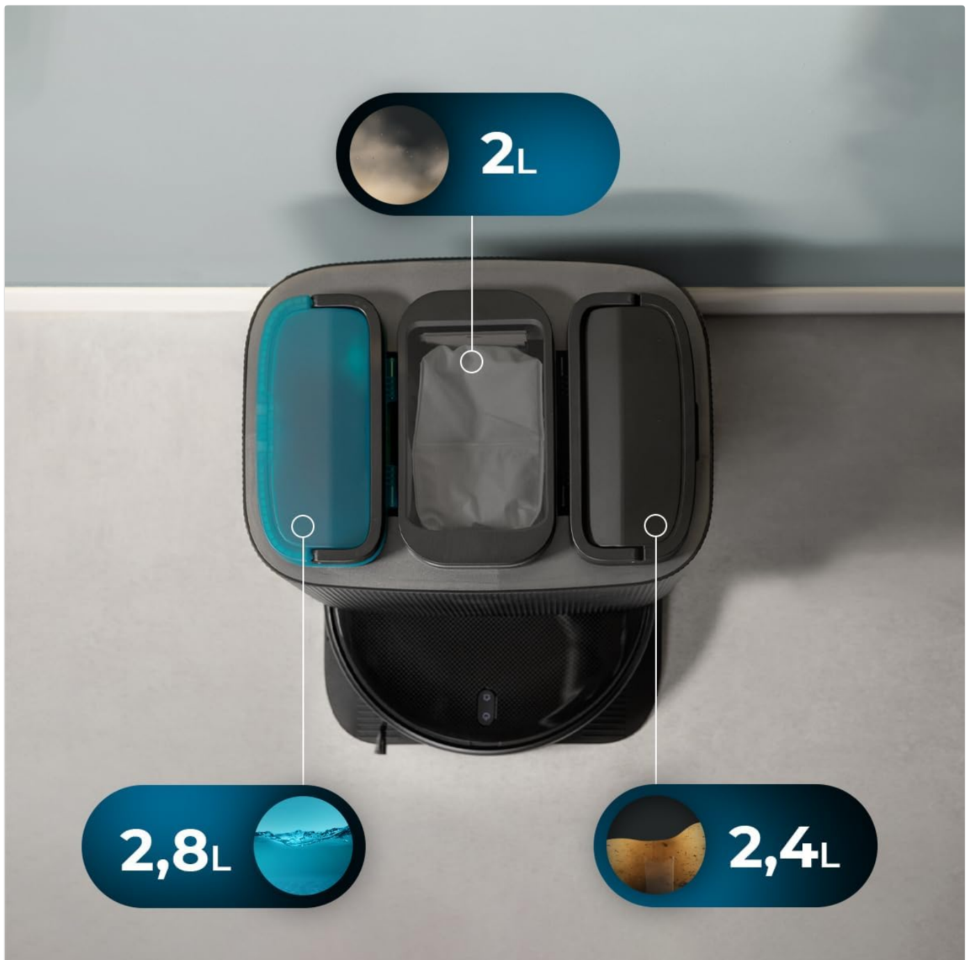
Figure 4.4: Overhead view of the station's tanks, indicating capacities for clean water (2.8L), dirty water (2.4L), and the dust bag (2L).
