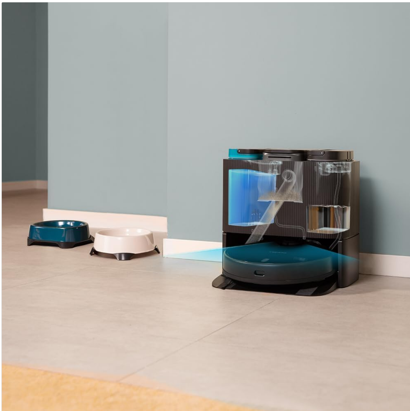
Figure 6.3: An internal view of the station demonstrating the process of dust collection and water circulation for mop cleaning.
