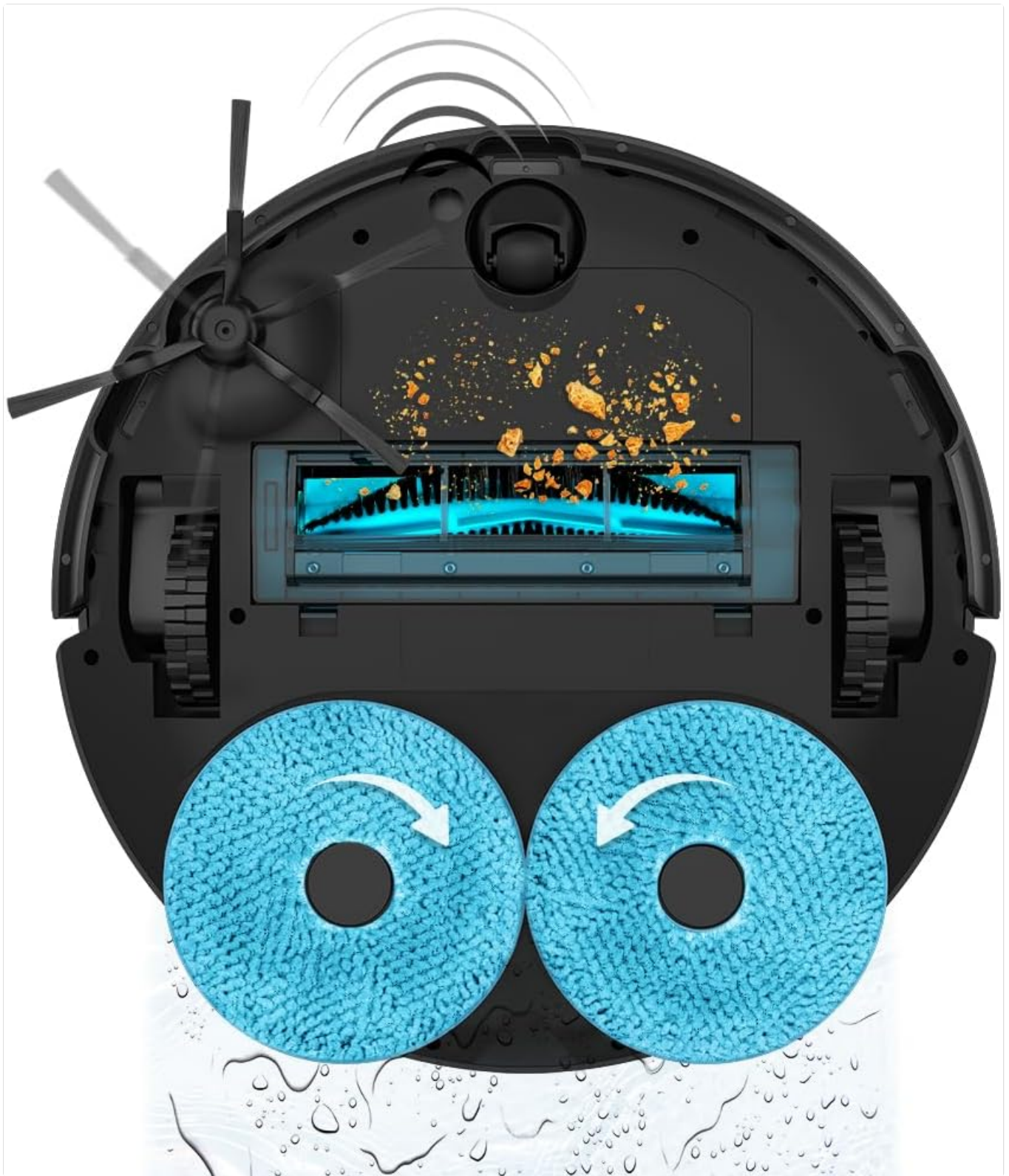
Figure 4.2: Underside of the robot, highlighting the main brush, side brush, and two rotating mopping pads.
