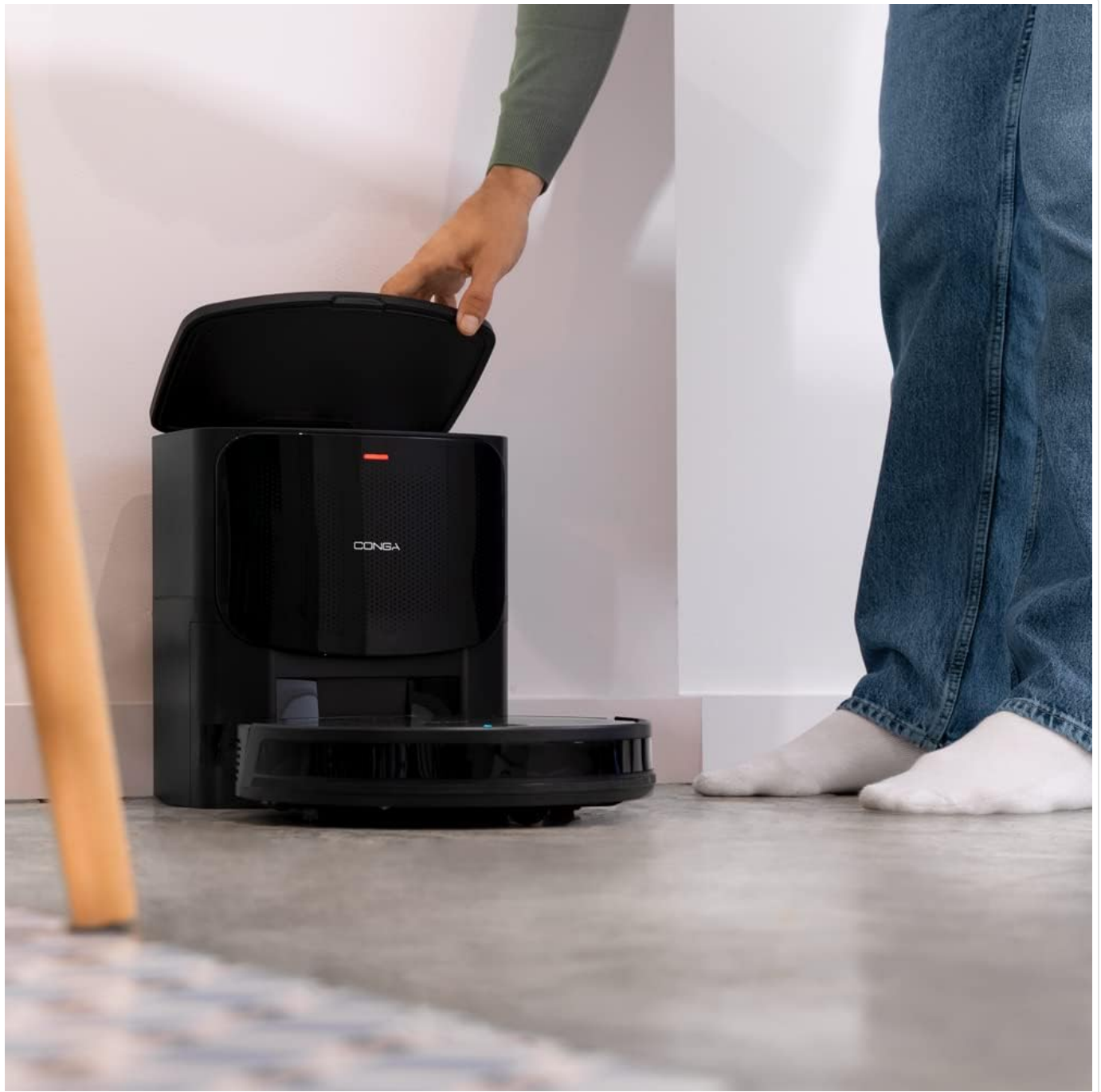
Image 5.1: A hand lifting the lid of the self-emptying base, revealing the compartment for the dust bag, indicating the process of maintenance.
