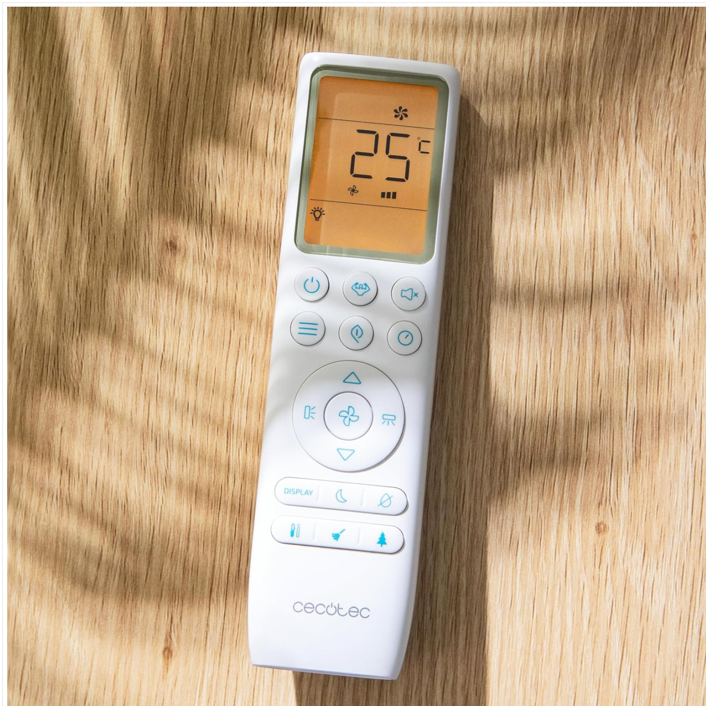
Figure 4.1: Remote Control. This image shows the white remote control with an orange backlit LCD screen displaying "25°C" and various function icons. Buttons for power, mode, fan speed, temperature adjustment, timer, and special functions are visible.
