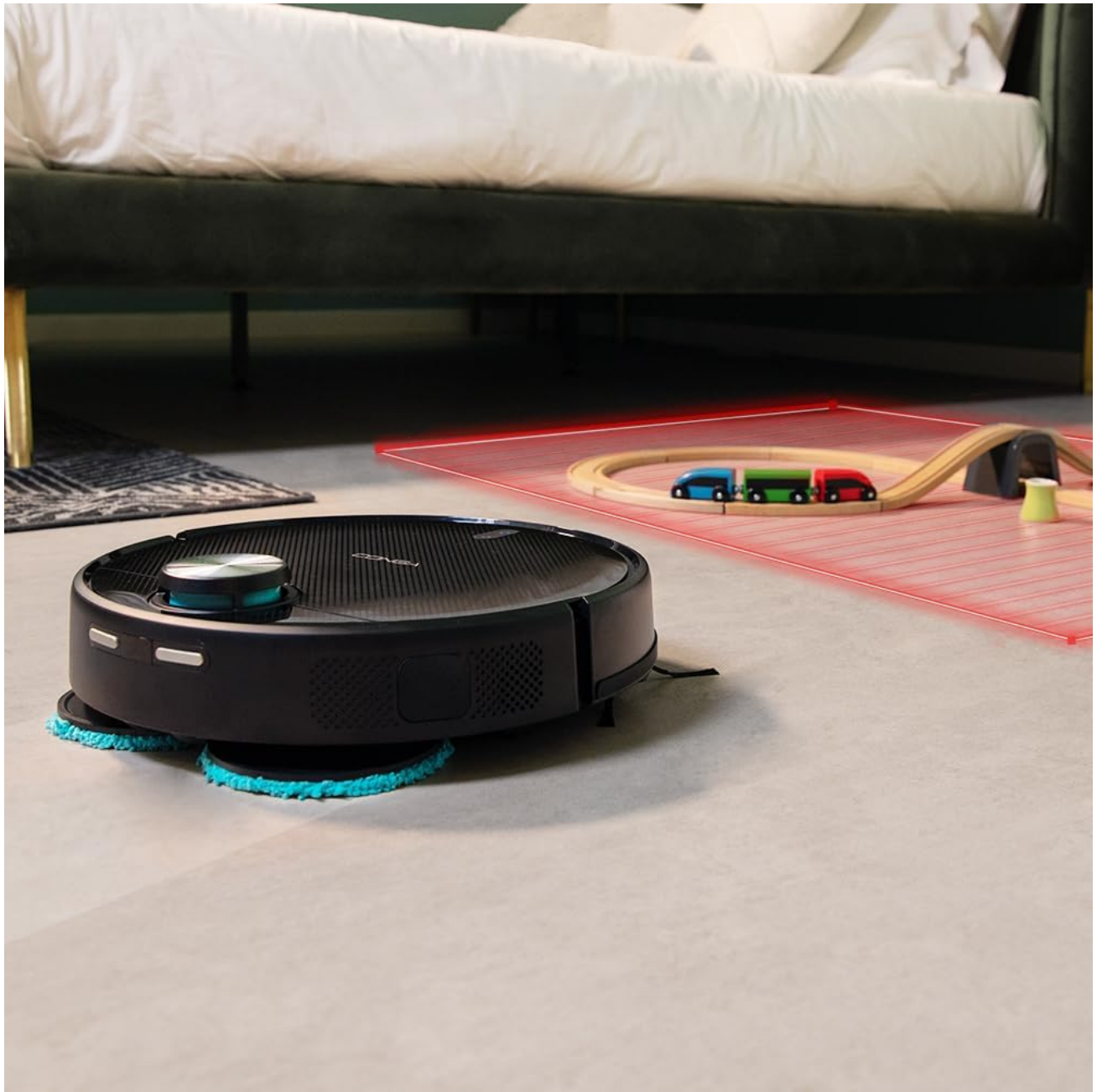
Figure 6.1: The robot utilizing its laser navigation system to efficiently map and clean the environment, avoiding obstacles.
