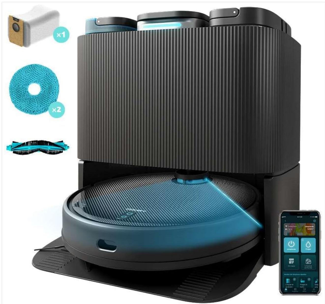
Figure 4.1: The Cecotec Conga 11090 robot vacuum cleaner docked in its self-emptying and self-cleaning base. The base features three compartments for dust, clean water, and dirty water.
