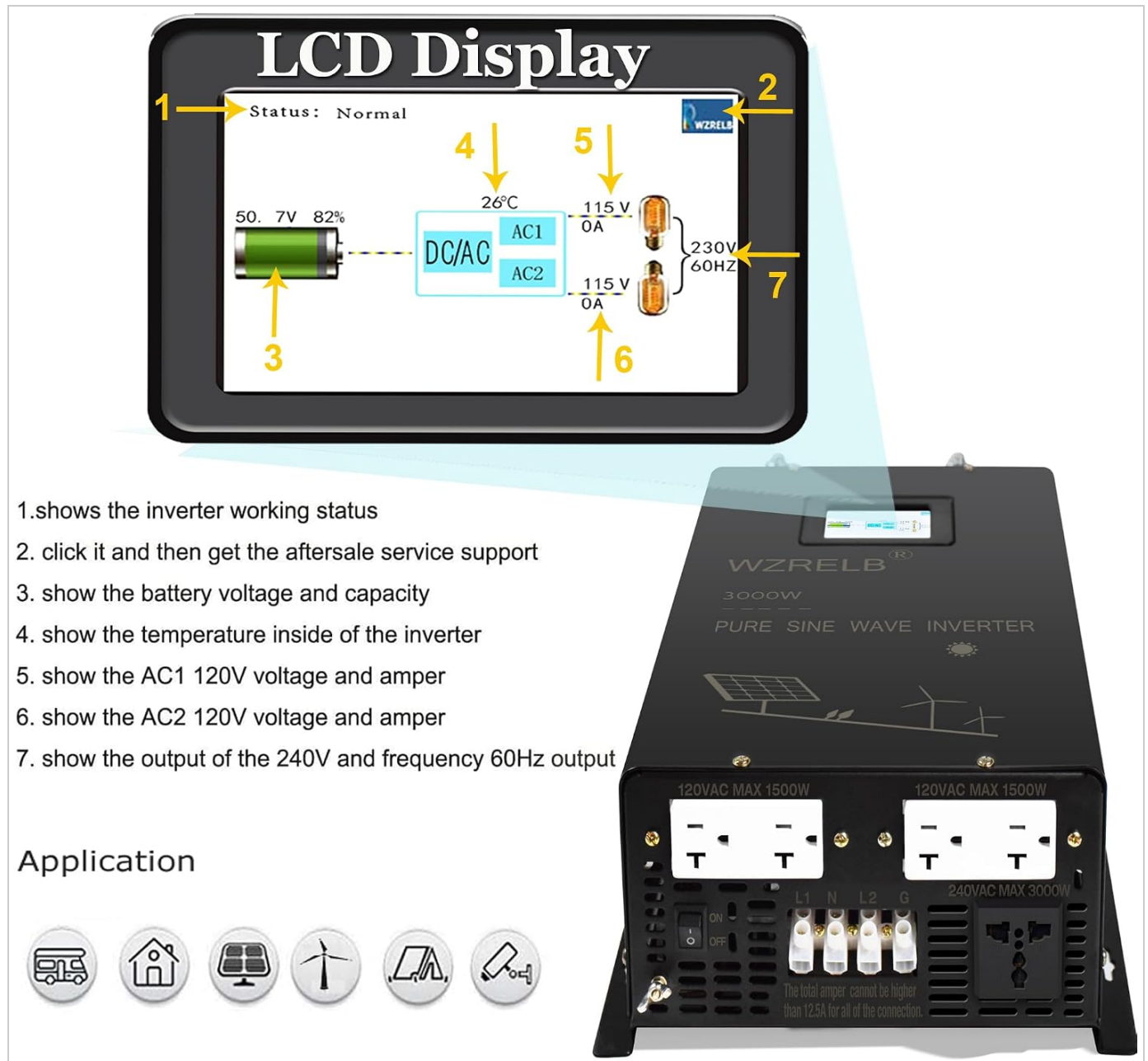
Figure 6: LCD display showing inverter working status, battery voltage and capacity, internal temperature, and AC output voltage/amperage for 120V and 240V circuits.
