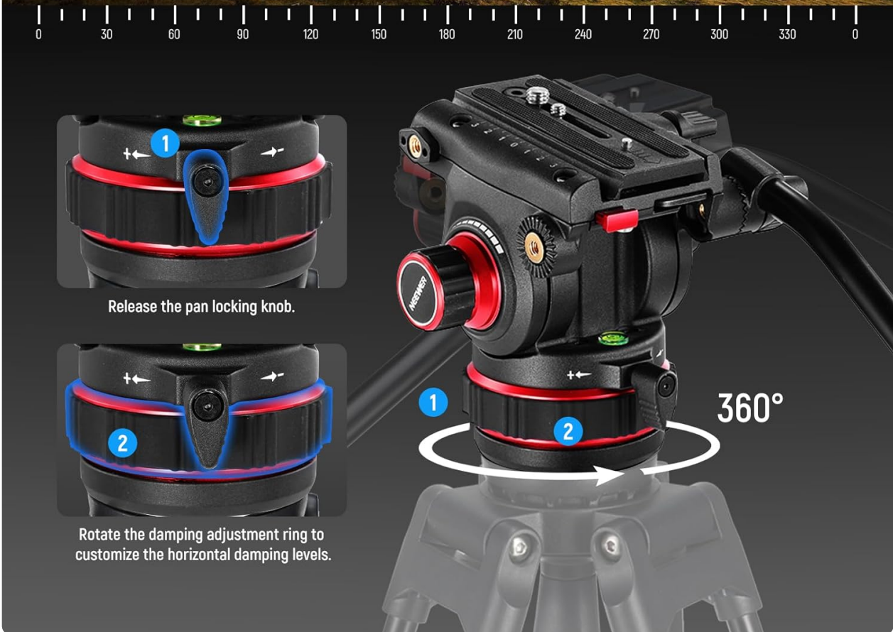
Image 3.1: Detailed view of the fluid head showing the pan locking knob and the panorama damping adjustment ring for customizing horizontal movement.
