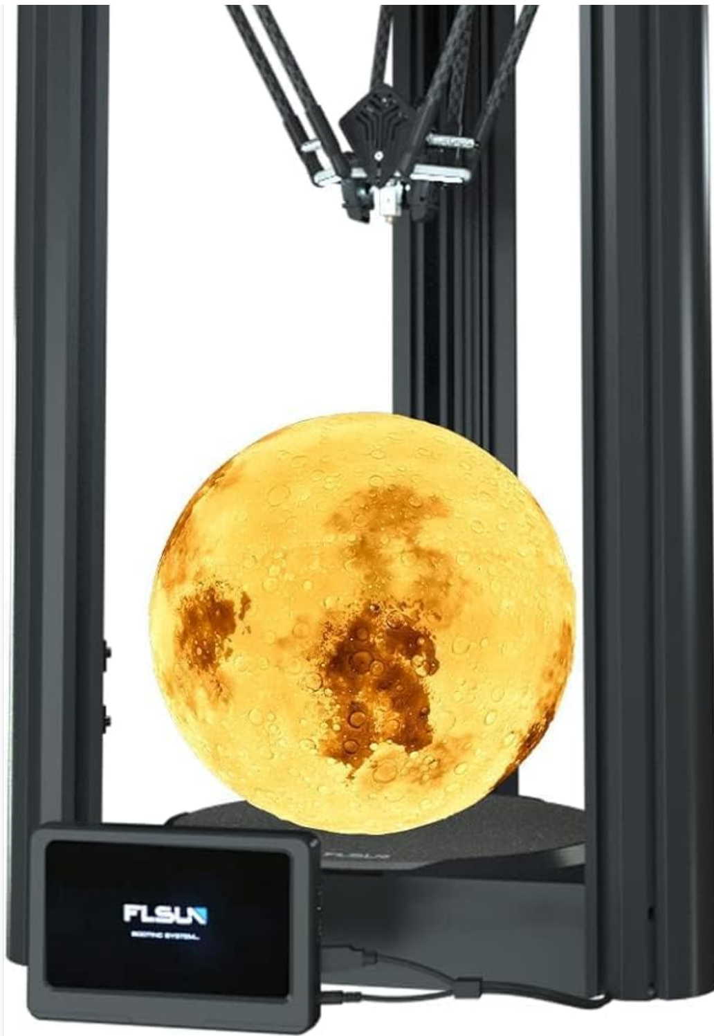
Figure 1: The FLSUN V400 3D Printer, showcasing its delta design and large build volume.
