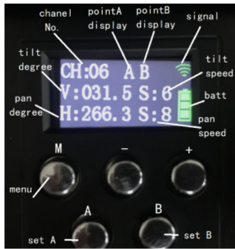
Figure 4.2: Control Panel Display.
