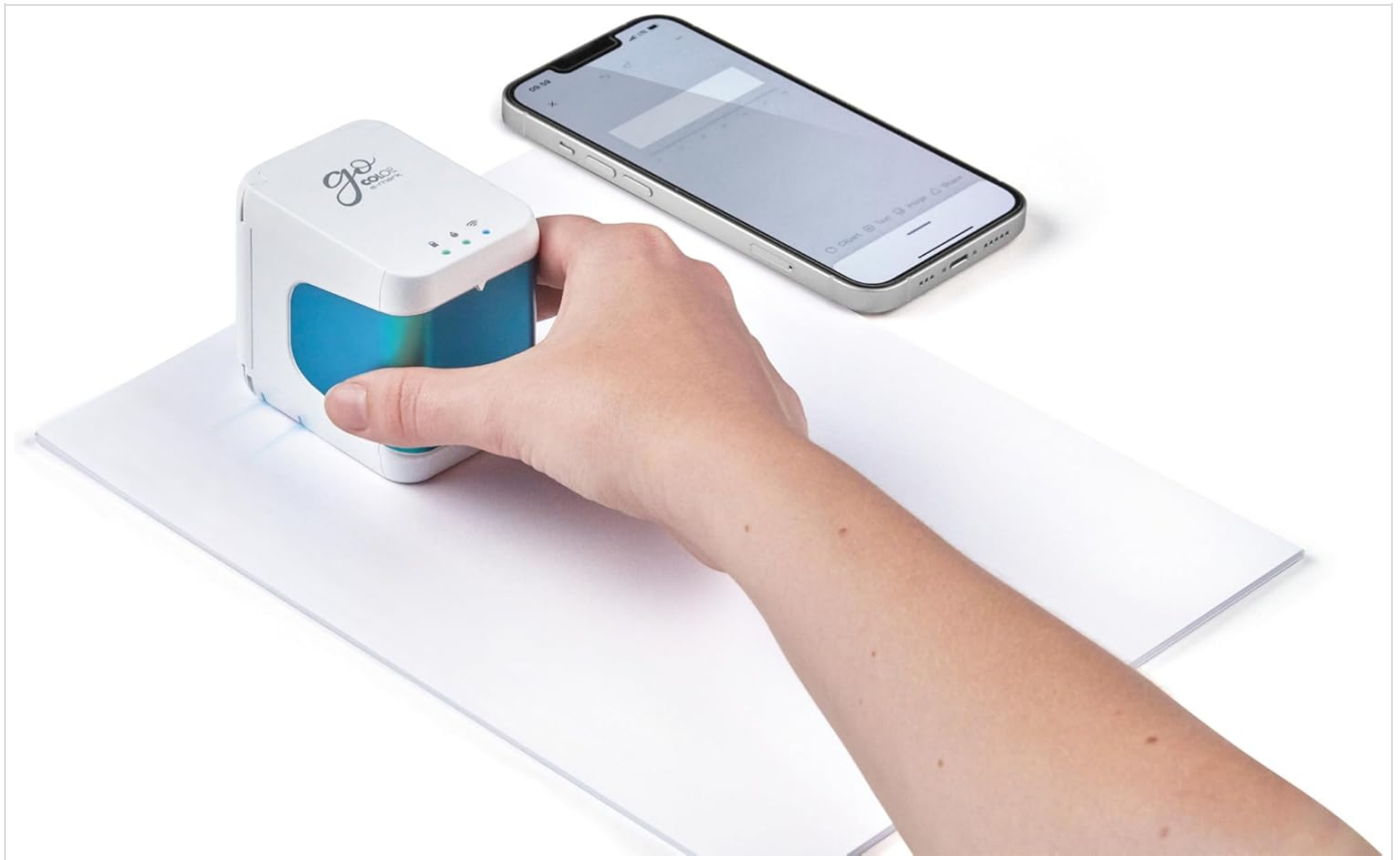
Figure 4.1: Demonstrating the printing motion of the e-Mark Go on paper, guided by hand.
