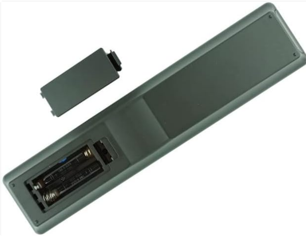
Image: Back of the remote control with the battery cover removed, illustrating the correct orientation for AAA battery insertion.
