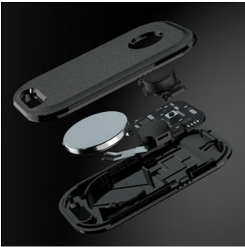
Image 5.1: An exploded view of the AIYATO Smart Air Tracker Tag, illustrating its internal components and the replaceable CR2032 battery.
