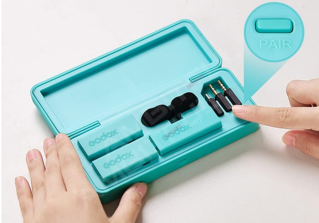
Figure 3: Pressing the PAIR button in the charging case.
