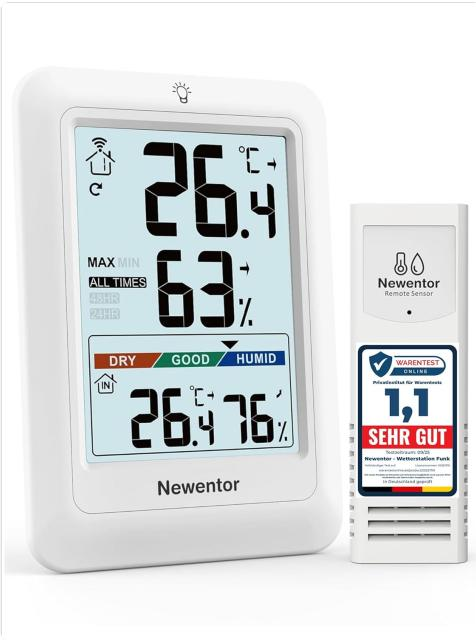
The Newentor Wireless Weather Station consists of a main display unit and a remote outdoor sensor. The main unit displays indoor and outdoor temperature and humidity, along with an air comfort indicator. The outdoor sensor wirelessly transmits environmental data to the main unit.
