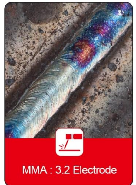
Figure 4: Examples of welding effects for MIG (CO 2 , MIX, Flux), Lift TIG (Metal Plate, Square Pipe), and MMA (3.2 Electrode).
