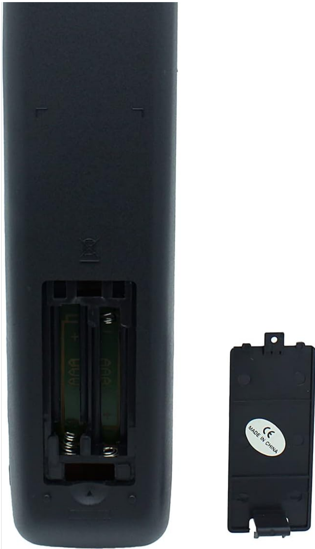
Image: Back of the remote control with the battery cover removed, illustrating the correct orientation for AAA battery insertion.
