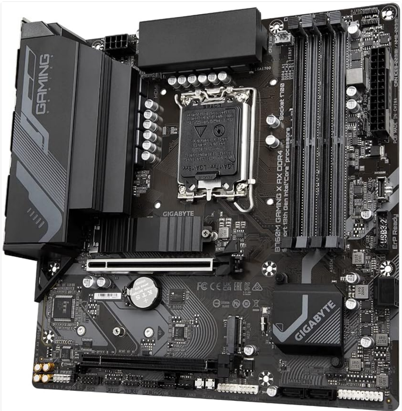
Image 2.2: Overview of the motherboard showing the four DDR4 DIMM slots.
