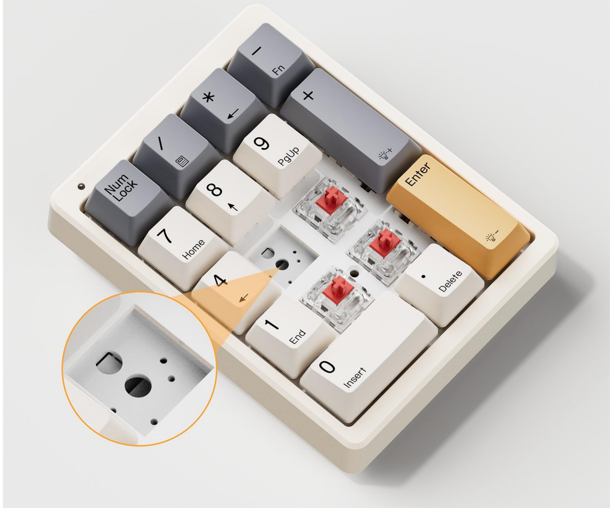
Image 6.1: Hot-swappable switch sockets on the PCB.
