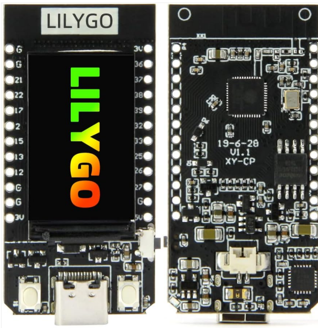
Image: Front and back view of the LILYGO T-Display ESP32 module board.
