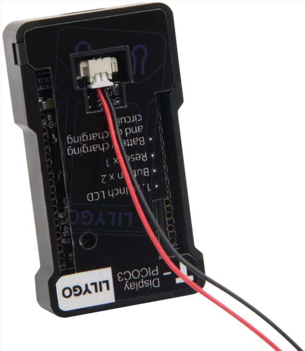
Image: The LILYGO T-Display ESP32 module with a Li-Po battery connected via its JST connector.
